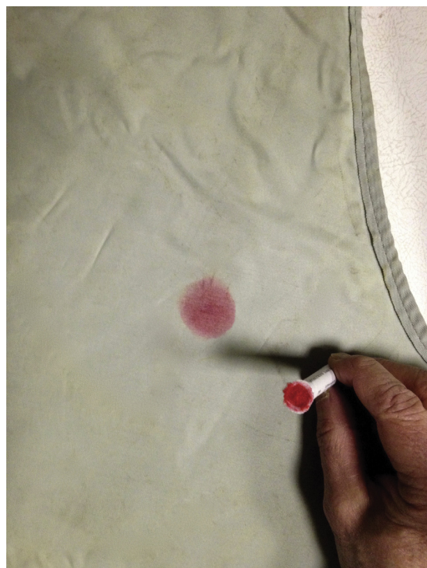
Fig 1. LeadCheck (3M) test performed on the upper right corner of a shield. Red color indicates the presence of surface lead dust. This red color was easily washed off with an enzyme-based cleaning solution.
